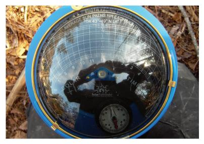
Harvesting heat from the sun is serious business in a Passive House, so the shading analysis must be accurate. The author relies on a Solar Pathfinder to determine shading conditions for the building site.
