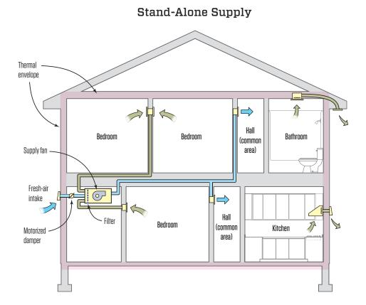
A standalone supply ventilation system uses its own fan to bring outdoor air into the house. To do it without comfort complaints, you'll need to temper the outdoor air before introducing it into the house, which you can do by mixing it with indoor air.
