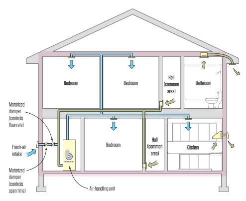
The central fan integrated supply ventilation system is the most common supplyonly system, especially in the humid Southeast.
