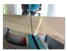
With a tall wood facing screwed to the fence, the saw can cut crown up to about  $3\,1/2$  inches tall in the standard upright, upside-down position.
