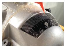
The saw bevels up to 48 degrees to the left, which is helpful when trimming out-of-square rooms.
