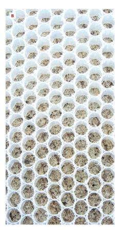
The hardware included in the kit can be used to install the Pro-Line linear drain on any floor surface, thin-bed, or thick mortar bed. The company's flat panels and sloping panels are made out of an innovative honeycomb material (8) and bond to the plywood or concrete subflooring (and to each other) with thinset mortar, which also fills the individual honeycomb cells for increased compressive strength.
