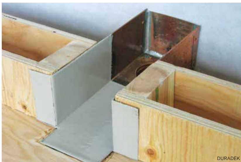
Figure 4. Thunderbird's 4-inch deck drain, designed for membrane-type roof coverings, is attached to 16-gauge copper flashing (top). The copper stair flashing in the center photo is just like deck flashing in miniature—when the cementitious deck coating is applied, it will completely cover the horizontal and vertical legs of the flashing. Duradek's copper scupper box (bottom) is coated with PVC so that the deck membrane can be heat-welded to it, making the assembly watertight.
