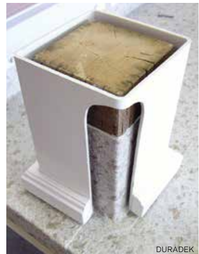
Figure 3. When wood posts must penetrate a roof deck, the flashing and roof covering are typically lapped up all four sides of the post and covered by a post sleeve.
