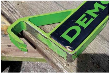
The Demo-Dek's sturdy steel jaw is sized to fit standard decking (above). The tool allows the user to stand on the existing decking (top), and doesn't rely on a joist for leverage.
