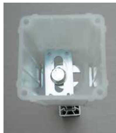
Figure 4. Vinylast's Plumb Perfect post and blocks are sold separately from the mounting kit, which includes a reinforcing base plate and four bolts (top). The top block on the Plumb Perfect post is adjustable up to \frac{7}{16} inch in any direction to account for the post being out of plumb, even after a post sleeve has been slid over the post (above).
