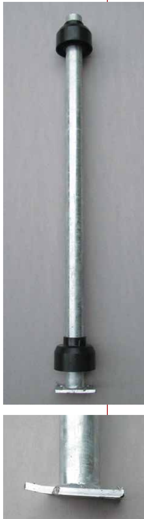
Figure 1. The EZ Post system doesn’t come with fasteners, an adjusting system, or a reinforcing base plate (top right). When fastened with 7/16-inch-diameter bolts and regular washers to doubled-up blocks that ran perpendicular to the rim joist, the washers and nuts began to pull through the blocking as soon as force was applied; at 373 lb., the blocking split, with more than a foot of deflection. When reinforced with another system’s base plate, the assembly was able to handle 500 lb. of tension, though the mounting plate bent (bottom right).
