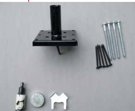
Figure 5. The Titan Post Anchor requires lag screws to secure the base plate to the post and 3-inch-long screws to fasten the base to the decking and blocking. Accessories such as a 1¼-inch-diameter hole saw (for drilling a mounting hole into the center of the post), a hammer cap, and a hole-saw centering tool are also available from Titan (above left). When the anchor was installed according to instructions, the inner screws pulled out of the blocking and decking at between 220 lb. and 270 lb. of force (above center). Using double blocking with the grain parallel to the tension force and through-bolts and washers instead of screws improved performance, but the top of the post deflected almost 12 inches (above right) before the bottom of the post finally split at 374 lb. of tension (right).
