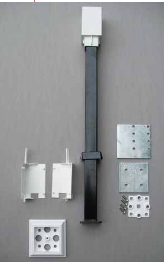
Figure 3. The UltiMount ProSpec kit comes with a galvanized surface plate and bottom plate, plumb adjusting bolts and nut plate, and a post-sleeve spacer and skirt (left). Not included are \frac{5}{16} -inch-diameter mounting bolts. While the reinforcing plates prevent the bolts from pulling through or splitting the blocks, the weld between the thin-wall steel post and the plate snapped at a little over 350 lb. (above).
