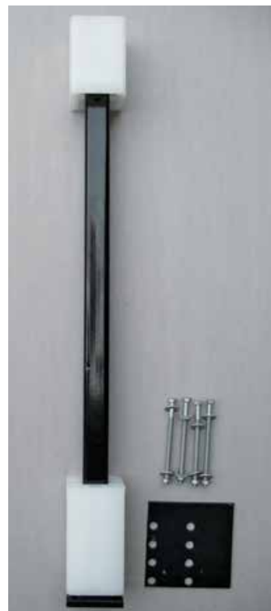
Figure 3. The UltiMount ProSpec kit comes with a galvanized surface plate and bottom plate, plumb adjusting bolts and nut plate, and a post-sleeve spacer and skirt (left). Not included are \frac{5}{16} -inch-diameter mounting bolts. While the reinforcing plates prevent the bolts from pulling through or splitting the blocks, the weld between the thin-wall steel post and the plate snapped at a little over 350 lb. (above).
