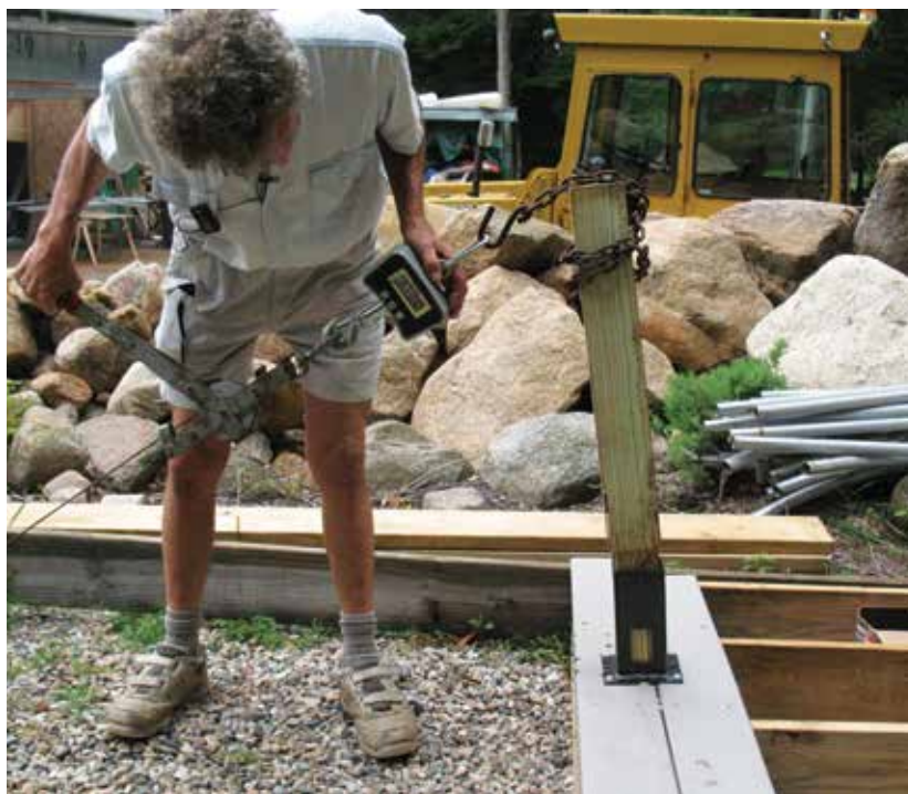
Figure 6. The Fiberon Post Sleeve Surface Mount kit comes with a heavy steel post box and plate, a rabbeted 4x4 post, and a concrete anchoring kit (left). The post base box stands 8 inches tall and bolts through double 2-by blocks with four \frac{5}{16} -inch-diameter bolts you supply. The author used the fender washers supplied with the concrete anchors to back up the nuts at the bottom of the blocking. The Fiberon mount had no trouble handling more than 500 lb. of force with only about 3 inches of deflection (above).
