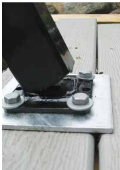
Figure 3. The UltiMount ProSpec kit comes with a galvanized surface plate and bottom plate, plumb adjusting bolts and nut plate, and a post-sleeve spacer and skirt (left). Not included are \frac{5}{16} -inch-diameter mounting bolts. While the reinforcing plates prevent the bolts from pulling through or splitting the blocks, the weld between the thin-wall steel post and the plate snapped at a little over 350 lb. (above).
