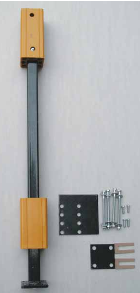
Figure 2. The TimberTech/Azek post is sold separately from the install kit, which includes an adjusting plate and adjusting screws along with a reinforcing bottom plate and bolts (top left). The top block has set-screw locations to lock onto the post for 36- and 42-inch-high railings. Anchor bolts drop through the holes at the corners of the base, while the smaller holes in the edges are threaded for the adjusting screws that are used to plumb the post (bottom left). The 3½-inch-square bottom of the post shows no signs of bending after testing at 500+ lb. of tension (above).
