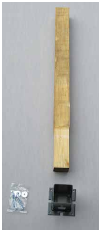
Figure 6. The Fiberon Post Sleeve Surface Mount kit comes with a heavy steel post box and plate, a rabbeted 4x4 post, and a concrete anchoring kit (left). The post base box stands 8 inches tall and bolts through double 2-by blocks with four \frac{5}{16} -inch-diameter bolts you supply. The author used the fender washers supplied with the concrete anchors to back up the nuts at the bottom of the blocking. The Fiberon mount had no trouble handling more than 500 lb. of force with only about 3 inches of deflection (above).
