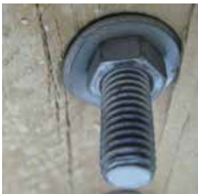
(D) When post kits were installed with bolts and washers rather than with a reinforcing base plate, the washers and nuts began to pull through the blocking long before test loads on the post reached 500 lb.
