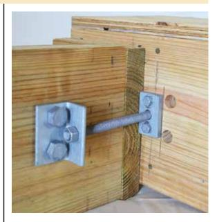
Deck-Con's Deck to House Connection Kit was designed to allow builders to install two 1,500-pound-rated connections between a deck ledger and house framing—without going inside the house. It can be used with dimensional-lumber house joists that run perpendicular to the ledger.
