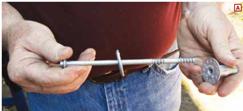
Figure 1. ThruLok screw bolts (A) provide a quick way to assemble built-up girders. They self-tap, like many wood screws (B), and are secured on the back with a wing nut (C).
