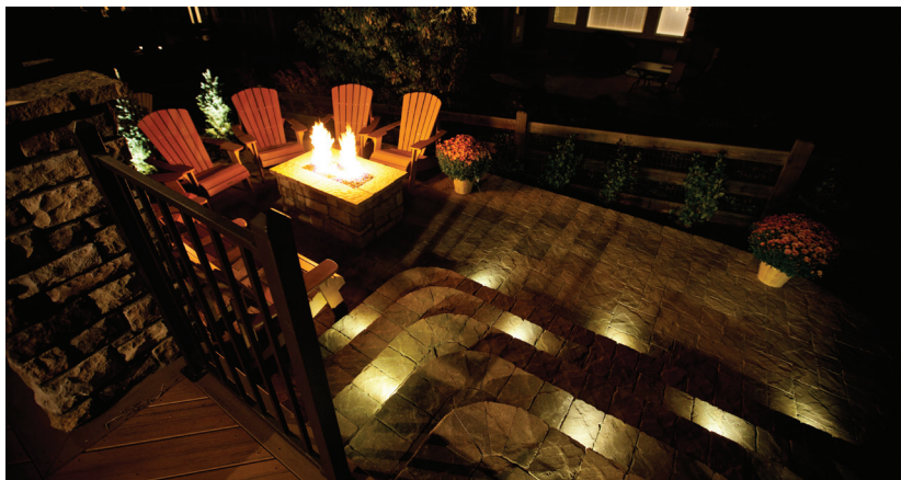
Step lighting is both a decorative element and an important safety feature when there is a change in elevation.
