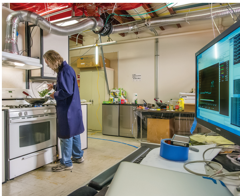
Researchers at the Lawrence Berkeley National Laboratory (LBNL) tested the exhaust efficiency of seven different kitchen vent fans with a variety of gas and electric cooktops.
