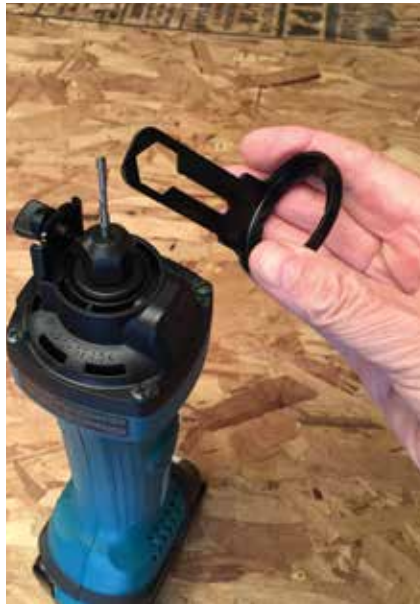
The router's adjustable shoe doubles as a collet wrench.
