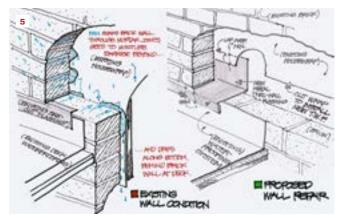
Modern brick fired at high temperatures can be fairly water-resistant. Older bricks are typically more porous and will absorb a surprising amount of water. But regardless of the type of brick, water will find its way through the cladding.
