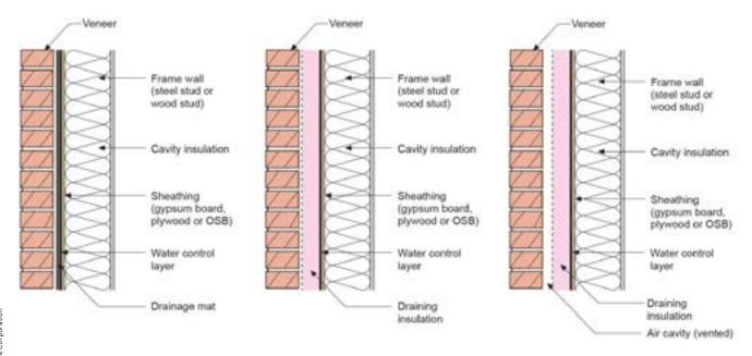
When using an advanced water-control layer, such as a self-adhesive or liquid-applied membrane, and a drainage mat or a draining insulation, such as mineral wool, no air cavity is needed. However, in IECC Climate Zone 5 and higher, and in areas with annual rainfall over 20 inches, a minimum 3/8-inch air cavity with vent openings top and bottom (far right) should be maintained.
