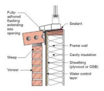
Self-adhesive and liquid-applied water-control membranes will reportedly protect the structural wall well enough that head and sill flashings can drain into the cavity instead of coming through the brick to the exterior face.
