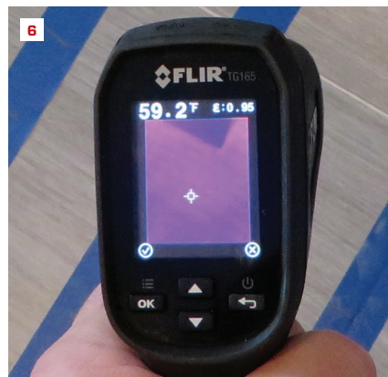
5. The Flir i7 autoranging has proven effective in use. The range can be manually locked. 6. The TG165 lacks a lock feature and the automatic ranging sometimes doesn’t show enough contrast.
