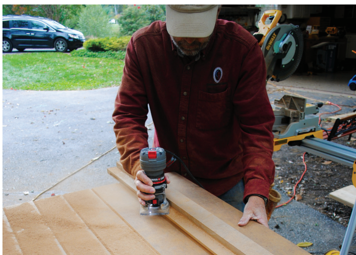
Figure 11. The author routed V-grooves in sheets of Extira panels, a weather- and insect-resistant product, for the finish back of the outdoor kitchen cabinets.
