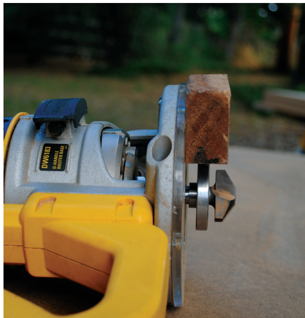
Figure 4. For routing the raised-panel design, a router was mounted with a bearing above the panel-cutting bit. A block of wood mounted to the base kept the router flat on the template.
