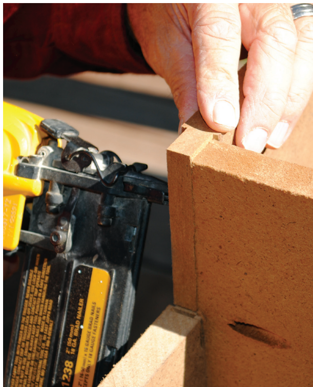
Figure 2. The bottoms of the cabinet boxes were sloped down from back to front to shed water. Also, the bottoms were cut \frac{1}{8} inch shy of the front of the cabinet-box sides to allow water to drip out.
