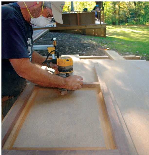
Figure 3. The author screwed together a template frame to guide his router during panel cutting. The screws could be removed to adjust the template for panels of different sizes.
