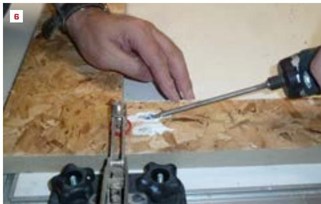
commercially available jigs for drilling the screw holes. We use a Kreg jig, which places the screws at a 15-degree angle to the face of the board. The jig clamps onto the back surface of the material being fastened and a specialized stepped drill bit with a stop collar creates the holes (2). We usually place one screw every 2 to 3 inches.
