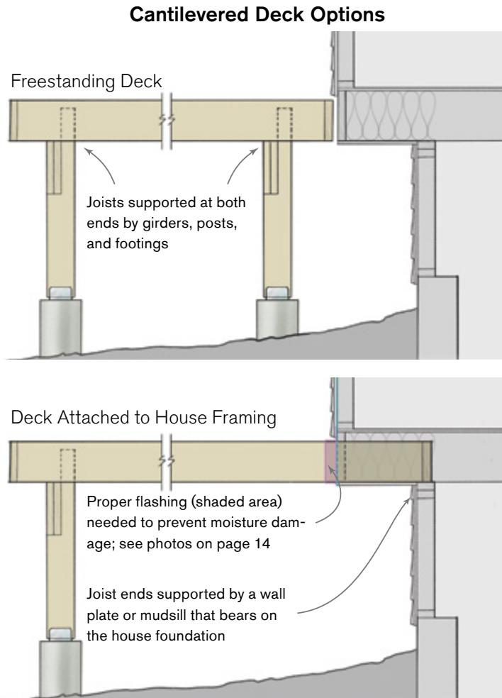
**A deck ledger cannot be attached to cantilevered house framing. Instead, build the deck either so that it is freestanding (top), or so that the deck joists extend into the house and bear on a wall plate or mudsill (above).**
