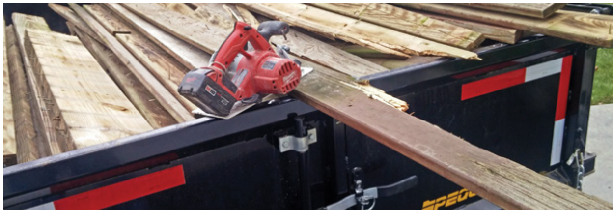
Figure 5. A cordless circular saw is handy for cutting old decking and framing to length so that it stacks efficiently in the back of a pickup truck or in a cargo or dump trailer.
