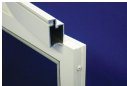
Figure 3. The aluminum frames for Connecticut Screen Works' commercial-grade panels have a .067-inch wall thickness and a 1-inch by 1 3/4-inch profile. The panels can be ordered in either fully-assembled or KD versions to fit openings as large as 16 feet by 16 feet.
