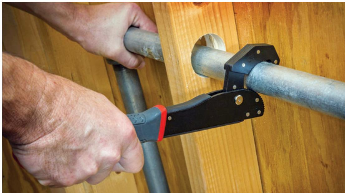
Crescent's 12-inch self-adjusting pipe wrench can be used like a ratcheting tool to quickly tighten or loosen rough-in plumbing and gas-line fittings from  $5/8$  inch to  $1\frac{1}{2}$  inches in diameter.
