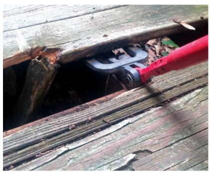
The angle of the Bull Bar's jaws can be adjusted by depressing the pin on the head and rotating the handle. When the pin is released, the jaws are locked in their new position.
