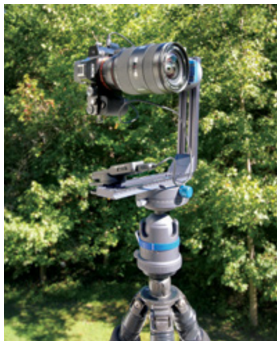
Figure 1. A mirrorless camera, such as the author's Sony a7R, has an electronic viewfinder that displays depth of field, exposure, and post-processing info before the shutter is pressed.
