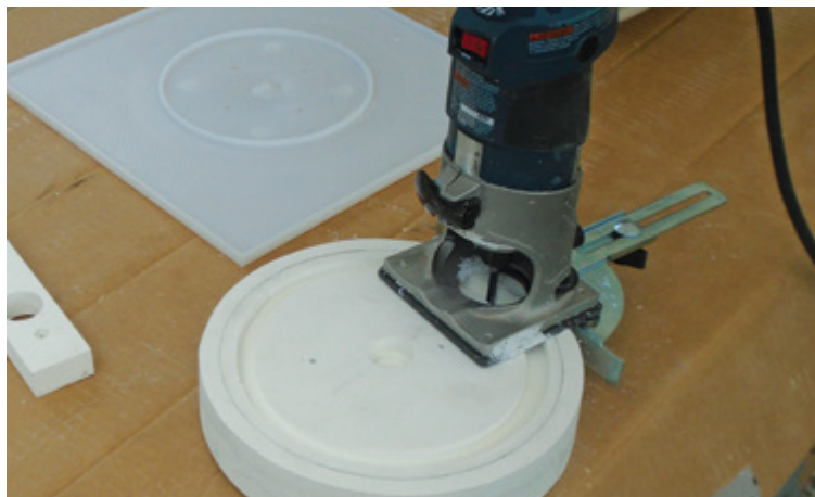
Figure 2. The author extended the columns by first inserting a plug made from a double layer of \frac{3}{4} -inch-thick PVC into the top of each column (above left). The plug serves as an attachment point for another, slightly larger PVC plug that's sized to match the outside diameter of the column and routed with a channel to fit into the flashing cap (above right). The column extensions effectively lower the position of the column's decorative trim rings.
