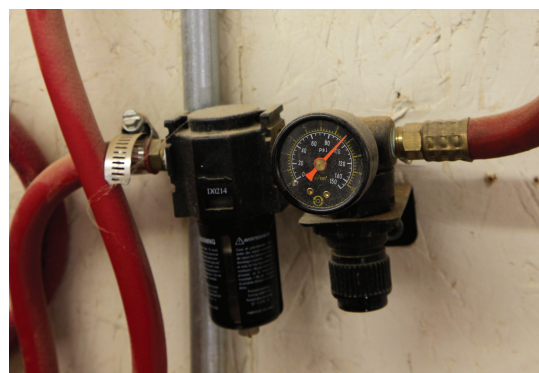
In-line pressure regulators are a convenient accessory for tools that require less pressure than the compressor provides.
