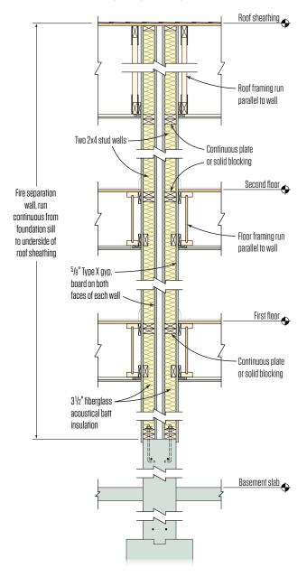
This classic example of a two-hour fire-rated assembly has two independent stud walls, each with fiberglass in the stud bays and  $^{5}/_{8}$ -inch gypsum board on both sides. Neither stud wall carries any floor load, but floor sheathing and ceiling wallboard are tied into furring secured to blocking in the wall.
