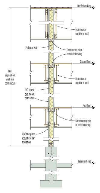
This typical one-hour fire-rated wall assembly uses just a single 2x4 stud wall with fiberglass in the stud bays and  $^{5}/_{8}$ -inch gypsum board on both faces. A one-hour fire-rated unit separation wall is allowed for duplexes, or for multi-unit buildings that are equipped with approved fire sprinklers.
