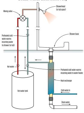
As warm water drains from the shower, it clings to the sides of a central drain pipe. Incoming water runs through tight coils around the pipe and recovers heat from the drain water. The warmed water then feeds the water heater and the shower.
