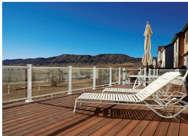
Either full glass panels (shown) or individual glass balusters can be used with the Fortress PureView powder-coated-aluminum railing system ( fortressrailing.com ).
