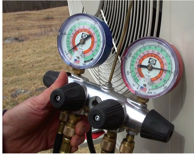
Technician David Ragsdale's pressure gauge shows the reading during a pressure test of the system at 600 psi (left) and during system evacuation at 170 microns (right) to purge moisture from the refrigerant lines.
