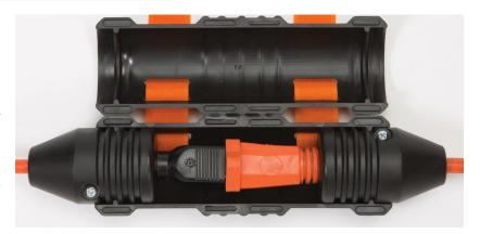
wraps around the stops, and Velcro straps lock everything together. The stops interlock with the shell so the cords can't be pulled apart. The shell also protects the junction and won't mar most finished surfaces. The system is compatible with after-market cord plug ends, as well. A
