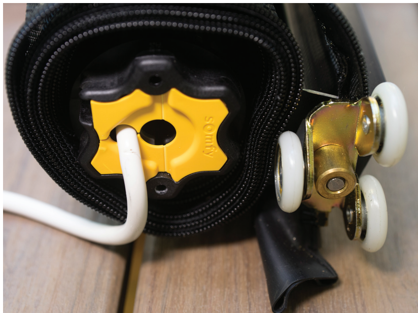
Figure 3. A Somfy tubular motor that can be inserted into either end of the rolled-up assembly powers the screen (top). A pin at the other end fits into the mounting bracket, while the bottom of the screen terminates with a heavy aluminum bar with rollers mounted to the ends (middle). A clip locks the assembly to the mounting bracket (bottom).
