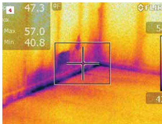
Combined with a blower door, an infrared camera can reveal cold air leaks. While the naked eye can see a water stain on the ceiling (1), the infrared image reveals the reason for the ice dam that caused it: heat loss through the ceiling and roof of the kitchen bump-out (2). In the bonus room over a garage, a cold wall and floor brought comfort complaints (3). The infrared camera revealed the cold air infiltration's leak point (4).
