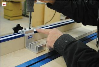
The stop system doubles as a measuring system for cutting on the miter-saw stand. To position the adhesive-backed measuring tape, slide the stop up to a board with a known length and mark the track (12). Place the tape with the length aligned with the mark (13), and then adjust the pointer on the stop until it's perfectly positioned (14).
