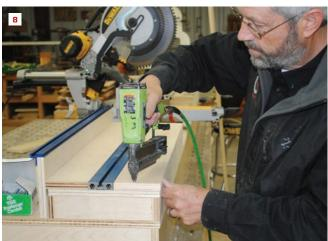
After building the platform and adding the support wings (1-3, previous page), lay out for the clamping track on top of the wing (4). Using a small section of track, mark out the bolt positions (5). After slipping the bolts through drilled holes (6), flip the top over and tighten the locknuts (7). Add strips on either side of the track for the final, flat wing surface (8).
