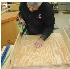
A lightweight storage shelf adds to the usefulness of the worktable. Pocket-screw the plywood frame together (19). Next screw the 2-by legs to the frame, using a framing square to keep them perpendicular (20). Position the shelf frame on spacers and screw it to the legs (21). Build the cantilevered saw platform out of 1/2-inch plywood (22).
