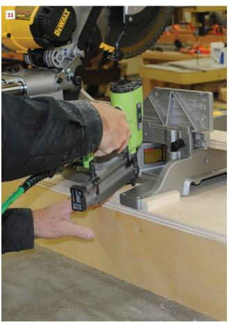
Using a straightedge, adjust the saw fence perfectly parallel with the wing fences (9). Extra space can be left to help with cutting crooked boards. Drive screws through each saw foot to hold it in place (10). Bolts and wing nuts replace the screws at a later time. Nail blocks around the saw feet to ensure perfect placement in the stand each time the saw is set up (11).
