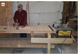
Screw 2x4 braces to the table frame to hold the saw platform (23), and screw the platform to the legs and braces with single screws (24). Put the saw on the platform and use a straightedge to align it with the table before attaching the platform permanently (25). A clamping plate added to the top increases the stand's usefulness (26).
