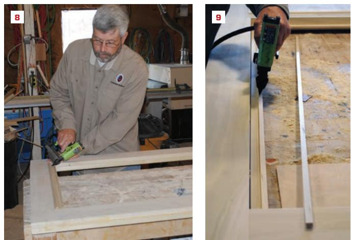
After the glue sets, a router with a flush-trim bit trues up the surfaces (5). The author tacks temporary blocks to hold the panel in the center of the opening (6) and attaches rabbeted panel molding to hold the panel in place (7). After pinning molding to the other side of the panel, he attaches the same molding to one side to hold the glass (8). To make up for the thickness difference, he attaches a thin strip to the back of the glass molding (9).
