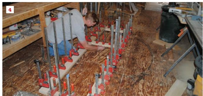
A story pole creates a full-scale layout for building the doors (1). After milling and cutting the parts, the crew assembles the frames in pairs. They roll glue on the frames (2), clamp the assembly at the corners, and place it on a flat surface (3). They add more clamps and wipe off excess glue with a damp cloth (4).
