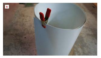
Spring clamps help to keep rolls of aluminum stock under control (5). Map out the bends for every shape and total up the dimensions (6). Mark the dimensions on one end of the stock and then fold the piece over on itself to transfer the dimensions to the other end (7). Short slits with tin snips register the dimensions on both ends of the stock (8).
