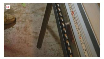
The two most common bends are the  $90^{\circ}$  and the  $45^{\circ}$ . The handle in the relaxed position is  $0^{\circ}$  (13). Bring the handle parallel to the floor for a  $90^{\circ}$  bend (14) and halfway to parallel for a  $45^{\circ}$  bend (15). "Hem" is the term used to describe material that's bent back on itself to make a finished edge (16). Hems are often part of another shape, such as this drip edge.
