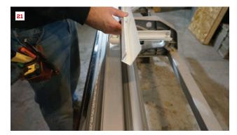
J-channel is a simple shape with two 90° bends (21). A drip edge uses two 90° bends, with a hem to strengthen the finished edge (22). On this modified drip cap, under-bending the leg that attaches to the wall adds a drainage slope (23). Casing shapes are also possible with a brake. This flat casing with a nailing flange is three 90° bends (24).
