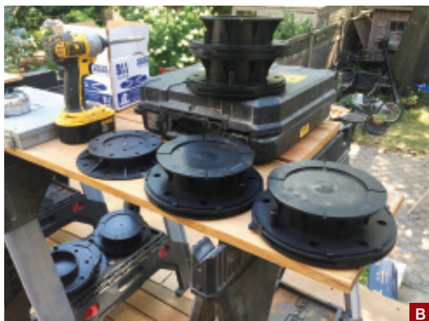
Figure 2. The 2-foot-by-4-foot ipe deck panels are flush with the top of the ipe curb and are supported by Bison Versadjust pedestals located at the corners and midpoints of the panels (A). To account for the slope of the roof, the author used different sizes of pedestals, each with a range of adjustment. The pedestals have angled bases that can be rotated to provide a perfectly flat surface to support the deck panels (B). During installation, spirit levels were used to level the deck panels, while tabs fitted to the tops of the pedestals provided the proper spacing between panels (C).
