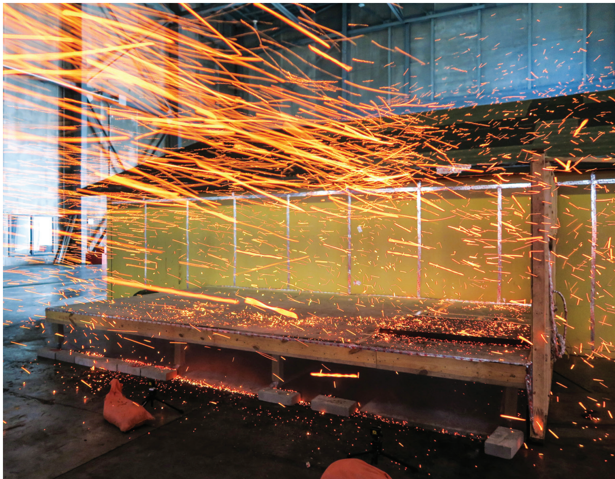
Figure 6. In testing conducted by the Institute for Business and Home Safety to simulate a wildfire environment, sample decks were exposed to windblown embers (which can start fires hundreds of yards from an active fire). Results showed that higher-density and solid decking were more fire resistant than low-density and hollow decking. Another key fire-resistant detail: Metal flashing that covers the first 6 inches of siding will help prevent windblown embers from building up at the intersection of the house and deck.
