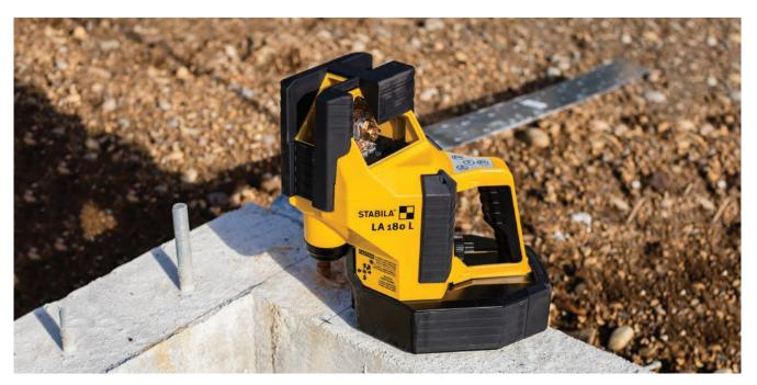
Many lines, many functions. The LA180L self-levels within 5 degrees, includes a 5/8-11 tripod mount, and can be affixed to a specialized saddle-type foundation bracket (sold separately for \$150). A control knob under the handle offers microadjustments for shooting square, but the unit can be auto-aligned with the REC410 Line RF receiver (included with the kit).
