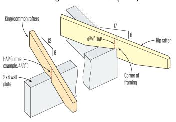
Hip rafters support the two sloping planes that make up a hip roof. Depending on the size of the roof, hips can be doubled or made out of different material, such as LVL. To keep the hip roof sections in plane with the main roof, the hip roof rafter must have the same height above plate (HAP) as the regular rafters. Measured at the common rafters, HAP is the vertical distance from the tops of the rafters to the plate at the edge of the wall framing.
