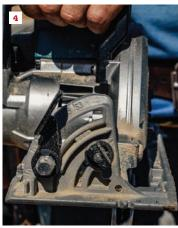
The Milwaukee M18 recip saw (1) performs better than any corded model the author has tried. And the DeWalt Flexvolt (2) actually cuts a little faster in thick material, but it's heavier. The Makita XSR01PT is powerful enough to compete with corded in-line saws. It has a large rafter hook, which tucks out of the way (3), and a table that tilts up to 53 degrees (4).
