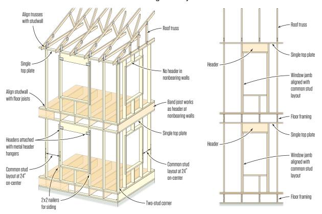
The illustration on the left shows the lumber-saving elements afforded by advanced framing, as they are typically rendered by advocates of the technique. On the right is a much more practical interpretation of an advanced frame wall, by architect Steven Baczek. This method maximizes the stud spacing but also will accommodate windows of varying size and position.
