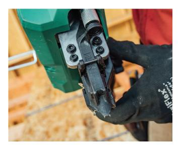
Good nose for toenailing. The nose design makes this nailer an excellent option for toenailing. The depth-of-drive dial is easily accessible, functions well, and is easy to follow while you're making adjustments.
