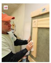
**Dust removal.** Even with a dust-collection system, a thorough cleaning is mandatory for a smooth paint job. The author first goes over the surface of the trim with a vacuum and soft brush (9). Then he wipes down all surfaces with a damp rag to remove any residue that the vacuum missed (10).
