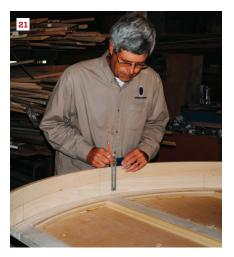
**Curved jamb layout.** The author positions one of the rails for the curved jamb on the back panel, measuring to a precise distance at all points (19). He then marks out the positions for the center stile (20), along with the positions for the side stiles. These marks also provide a side-to-side index of the rail to the back panel for aligning after the arched jamb is assembled. Stacking the second rail on top of the first, he draws the marked positions on both curved rails (21).
