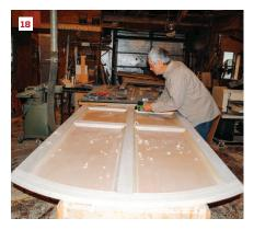
**Trimming out the back panel.** To apply the panel moldings to the back, the author first scribes the curved intersection of the molding using a short scrap (16). This allows him to measure and cut the intersecting angles precisely. Clamps hold the curved moldings in place while he nails in the rest of the panel molding around the top sections (17). Panel molding around the bottom sections completes the back panels (18).
