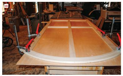
Assemble the back panel. To build the back panel, the author first scribes the tops of the stiles to the curved top rail (13). Pocket screws and glue connect the frame pieces for the back panel (14). When the panel frame is assembled (15), the author cuts the tails off the curved top rail. He then glues the frame to the plywood back, flips the assembly over, and cuts off the excess plywood with a router.
