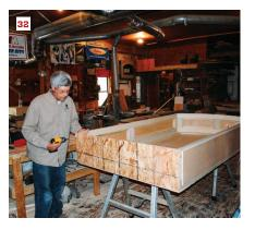
**Attaching the side jambs.** The author positions the sides of the niche on the back and clamps them in place. He then attaches the sides with screws driven from the back (30). Before joining the top to the sides, he aligns them with a framing square to make sure they join at a precise right angle (31). To keep the bottom of the niche stable for cutting the trim and for transportation, the author screws a piece of OSB to the bottom edges of the sides and back (32).
