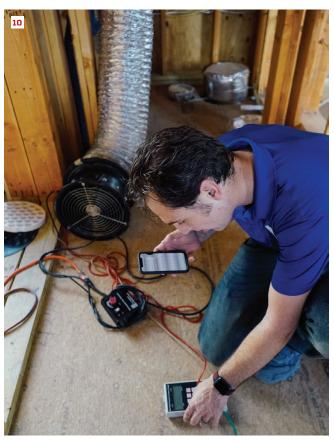
After hooking up the Duct Blaster, Harris adjusts the fan controls to bring the pressure in the system to 20 pascals (8). By itself with no-air handling equipment hooked up, the duct run is remarkably airtight—so airtight that to get meaningful numbers, Harris has to insert a "Ring 4" flow restrictor into the fan assembly (9). With the flow restrictor in place, Harris recalibrates the pressure and flow gauge, and uses his smartphone to calculate the equivalent leakage rate.
