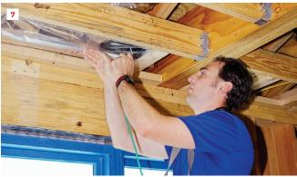
To prepare for pressure and airflow testing, Harris attaches the Minneapolis Duct Blaster's collar to the end of a supply duct, sealing the inside of the collar (5) and the outside with tape (6). Next, Harris inserts the end of the Duct Blaster manometer's pressure-sensing air tube into the taped-off end of the duct (7). When the fan is up to speed, the device's DG-700 pressure and flow gauge will calculate the duct run's air leakage.
