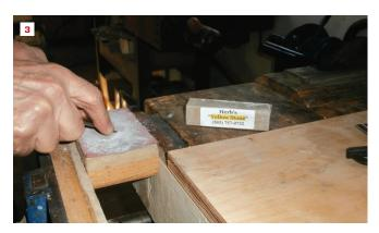
To tune a plane, the author starts by flattening and polishing the sole on a sheet of sandpaper taped to the bed of his jointer. Roll or break all the edges of the plane body (1). After grinding a 26° to 30° bevel on the iron, the author hones the edge on a whetstone to the same angle (2). The last step is stropping on a piece of leather (rough side up) tacked to a block and loaded with Herb's Yellow Stone compound (3).
