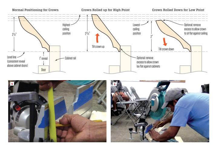
When the crown molding lands within an inch of the tops of the cabinet doors, an out-of-level condition can often be dealt with by rolling the crown. For this  $2^{1}/2$ -inch crown, draw lines on the miter saw fence at 2,  $2^{1}/4$ ,  $2^{1}/2$ , and  $2^{3}/4$  inches (see illustration and photo 4). For crown that is only 2 inches high, set the edge at the 2-inch mark and cut the miters at 45 degrees (5).
