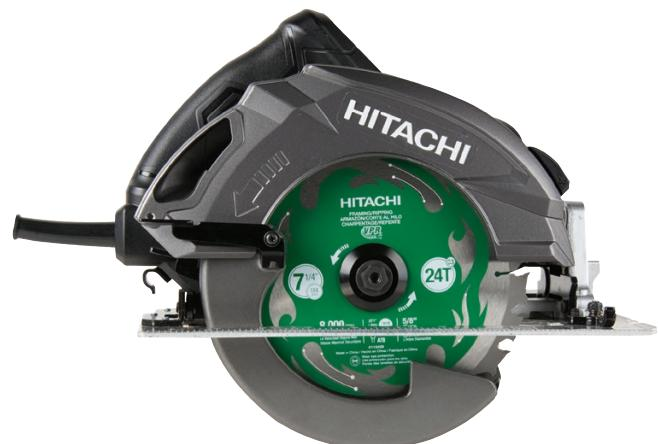
**Two versions available.** The RipMax is available with or without an electric brake. Both versions have the same features otherwise, though the non-brake model (C7UR) can bevel up to 55 degrees, whereas the electric-brake model (C7BUR) is limited to 45 degrees due to a larger motor housing. Both saws weigh just slightly over 11 pounds.
