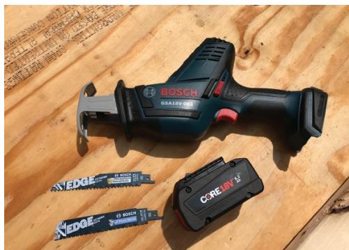
The Bosch GSA18Vkit comes with a 4.0-Ah FatPack battery. But for a lot of his work, the author ran it with a 6.3-Ah Core battery, which performed exceptionally. On most jobsites, a reciprocating saw is used in short bursts, allowing the tool and battery to take a break and cool off. One battery is usually enough.
