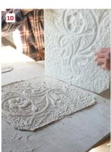
Ron trims the wax negative (5), while William and apprentice Derek Dawson mix fast-drying gauging (gypsum) to make the bottom, or saddle, of the mold (6). After the wax has been sprayed with oil, the gauging plaster is poured over the wax (7), flattened (8), then later flipped over (Hydrocal is used to make the new pieces). First, the mold's saddle is removed (9), then the paper-thin, Hydrocal replacement piece (10).
