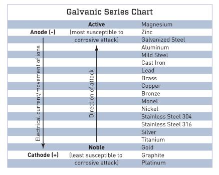
This chart lists common metals in order of how reactive they are with other metals. The greater the distance between two metals on the chart, the greater the potential for corrosion when they're in contact.
