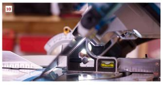
Set a square against the table and press it lightly to the blade (7). Shine a light behind the square (8). If the saw has a detent plate (9), setting the blade square to the table will account for other detent angles. On some saws, you have to set the 45° stop independently. A combination square works well (10).
