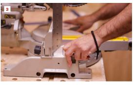
Check for flat, straight, and square. The table should be flat, with no high or low spots. A thin straightedge like a framing square is better here than a level because it makes identifying the location of potential trouble areas easier (1). Remove the auxiliary fence from the stationary fence and check it for straightness, adjusting as needed (2). Replace the auxiliary fence and check that it is square to the table (3).
