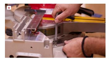
With the saw's head set at the 90° detent, clamp the try square to the saw blade so that the square can register near the top of the fixed fence. A flashlight will help identify even the tiniest gaps here (4). Loosen the miter plate screws and gently tap the end of the table until the light disappears (5). Lock the head in place and then tighten all the screws on the detent plate (6).
